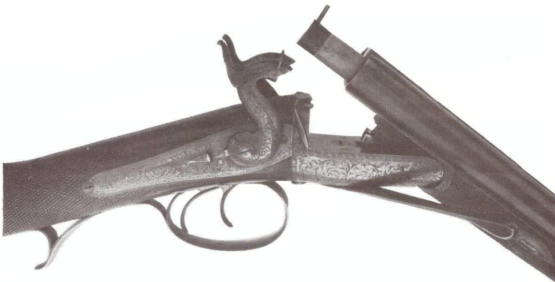
Double barrel early pin-fire rifle made by Joseph Lang showing early form of breech action and cartridge, c. 1858.
