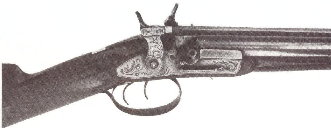
Double barrel tube-lock gun made by Joseph Manton, c. 1818. Barrels of the Manton tube-lock illustrated below bearing the initials of Charles Lancaster, who forged them.
